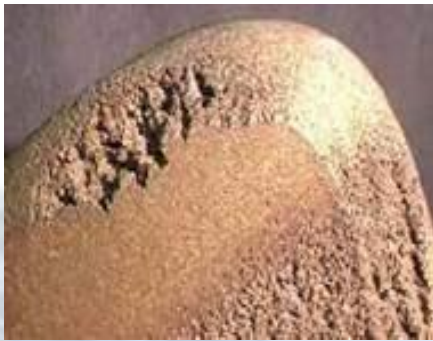
Metal Destruction from Uncontrolled Cavitation
