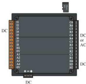
VCS (VRTX Control Station). Always connected to VDC, V+/- on the power connection and Input (orange) block, however the output (large black connection can be VAC or VDC powered and you need to see what is connected to understand if it is AC or DC for testing.
