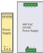
Power Supply. The bottom Inlet is always Volts AC, V~ while the output is always VDC, V+/- . Normally the input is 120VAC or 480VAC as shown on the power supply. The output is always 24VDC V+V-. The smaller white units are 120VAC input while the larger silver one is 480VAC.
